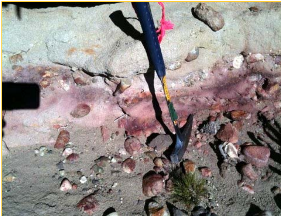
Image 4. Close up view of the above photo showing the Los Adobes conglomerate displaying purple-red hematite alteration characteristic of sediments within the oxidized portion of a roll front system.
